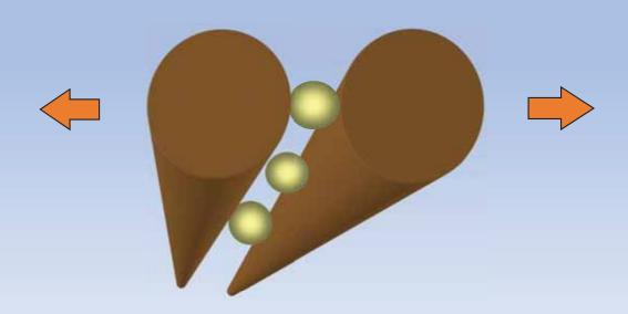
Contact Angle  $> 90^{\circ}$  causes the fibers to be pushed apart
